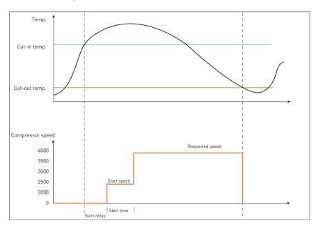
If the compressor speed drops below the minimum or exceeds the maximum speed, the compressor will stop and an alarm **Min speed failure or Max. speed failure** will be sent. The compressor will try to restart after the set **Restart time**. The **Restart time** default is 60 sec The fans will continue to run.
